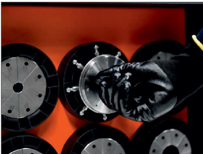
Picture 3: Picking the die set from the cabinet
